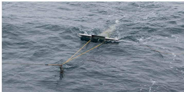
Fig. 6.1: Manta Trawl (MT) deployed in the Southern Ocean. Between the yellow bridle of the MT and the steel rope of the on-board crane an 8 kg steel weight is attached to stabilise the trawl.
