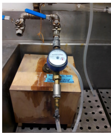
Fig. 6.2: Wooden protection covering geological sieves to allow for undisturbed sampling. Samples are taken from the on-board seawater intake system connected to the protected sieve stack with a water meter and a silicone hose.
